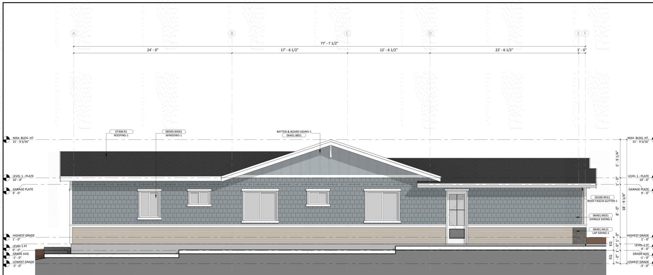
0 2' 4' 8' EXTERIOR ELEVATION - NORTH SCALE 1/4" = 1'-0" 2
