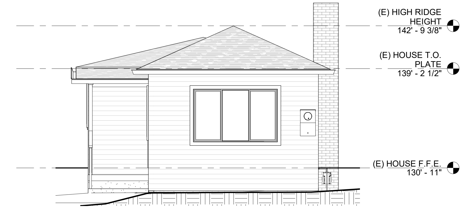
1 EXISTING FRONT ELEVATION 1/4" = 1'-0"
