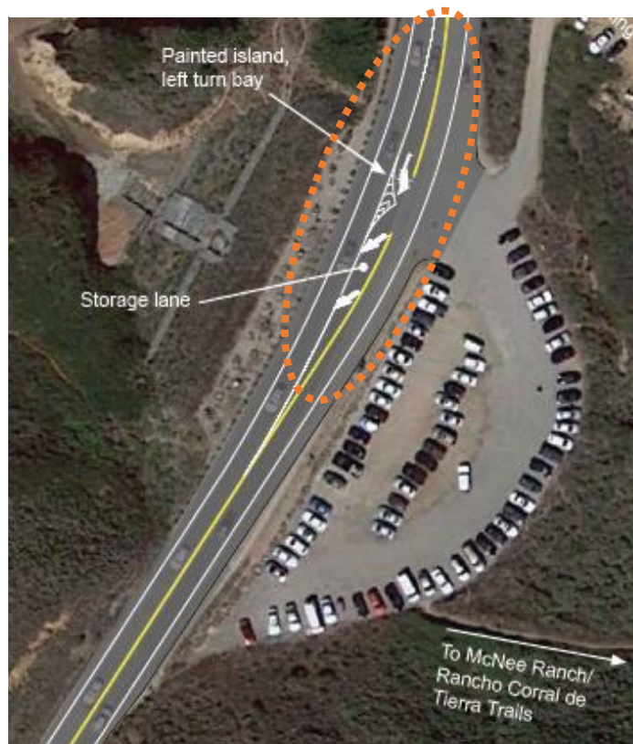
Figure 6: R3. Gray Whale Cove Turn and Acceleration Lanes Concept Diagram
